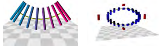
Figure 7: A polyscrew obtained through 4-point subdivision from only two control poses produces a smooth pendulum motion (left). A polyscrew obtained through B-spline subdivision from four control poses (in red) produces a spinning motion of a block (right).
