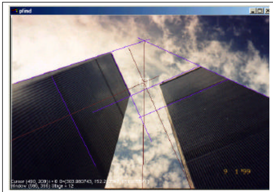
Fig 7: The purple lines are the user-selected lines, the maroon lines are the altitudes of the vanishing point triangle, and the white box encircles the calculated image center (where the altitudes intersect).
